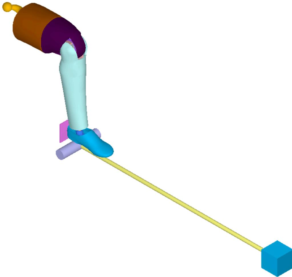
Figure 19. Setup of the lower foot impact test.
