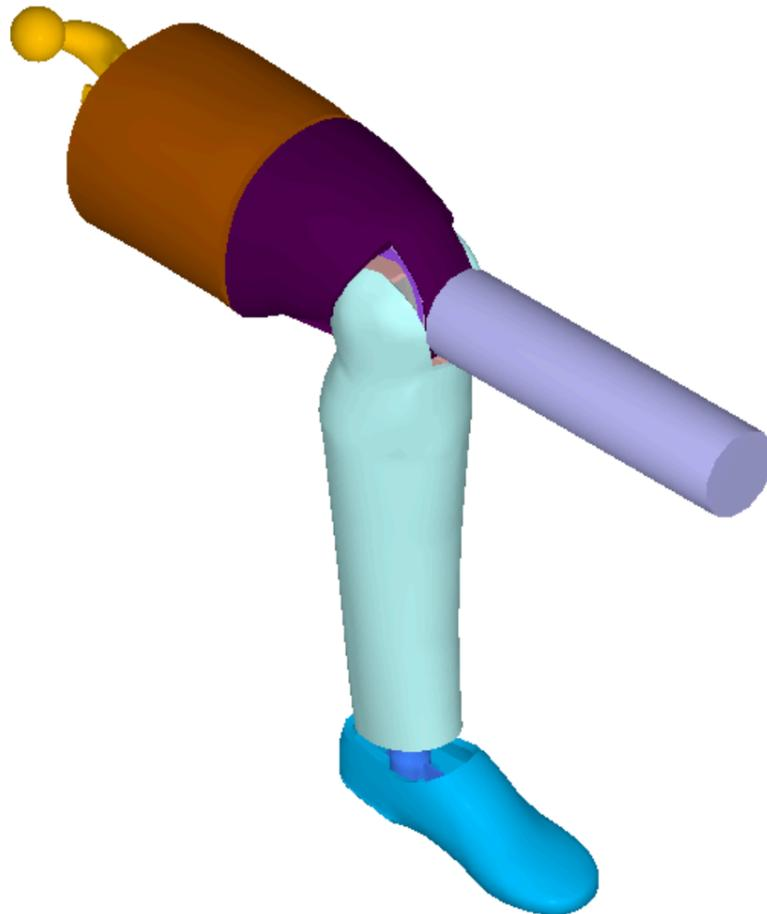
Figure 13. Setup of the knee impact test.
