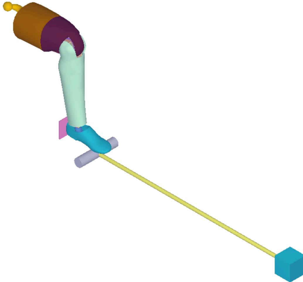
Figure 17. Setup of the upper foot impact test.
